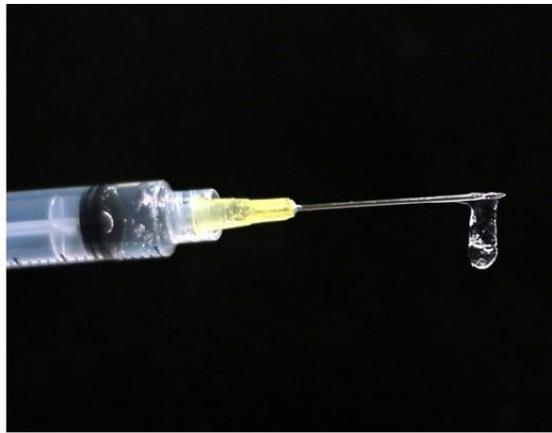
*HyStem* hydrogel extruded through a 20-gauge needle
